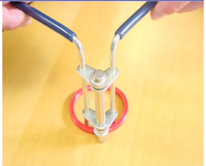
Kidney shape the u-cup seal by closing the arms of the installation tool. Be sure not to overstress the seal during kidney shaping. Thicker cross-sectioned seals will be more difficult to kidney shape.
